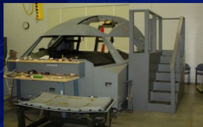
Crew Escape System Maintenance Trainer (CESMT) - 1
